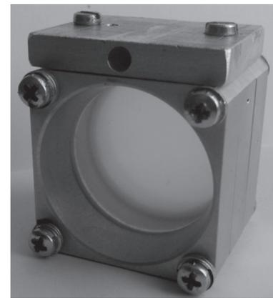
Fig. 2. – Measurement cell for research of ferromagnetic fluids in quasi-optical beams.
